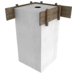
Foundation concreted on-site
