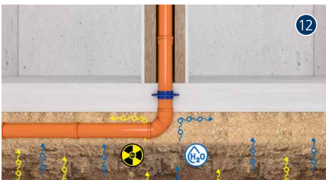
KGF110 set in concrete
