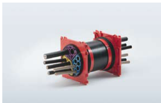
Fig. 5 Use of the Segmento system for up to 24 cables with a max. diameter of 15 mm each at a watertightness of up to 5-m water column.
