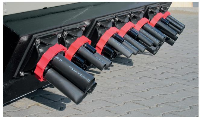
The chloroprene surface sealing fits perfectly to the building entry sealings of the station. Thanks to the cathodic dip coating of the aluminium flanges a optimal corrosion protection was achieved. Sealing of the cables is done by means of heat shrinkable sleeves. Not used openings will be safely closed with a blind plug.
