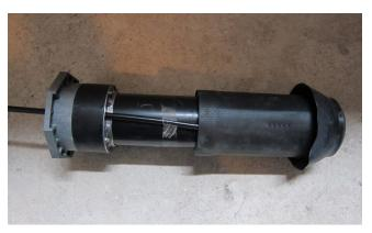
Adaptation of the building entry to the on-site conditions: cutting to length and adaptation to wall thickness. Sealing is achieved through injection of a 2-component resin via a filling hose.
