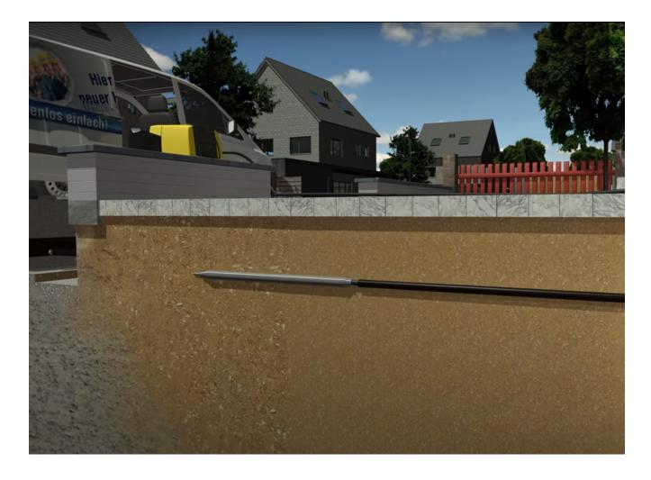
TRENCHLESS BUILDING CONNECTION FOR BUILDING WITH BASEMENT
