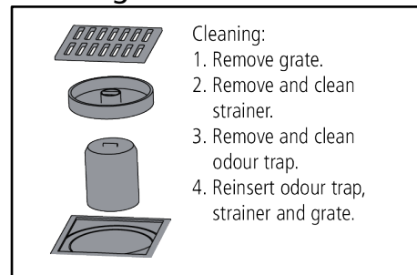
Cleaning Version without backflow preventer 1
