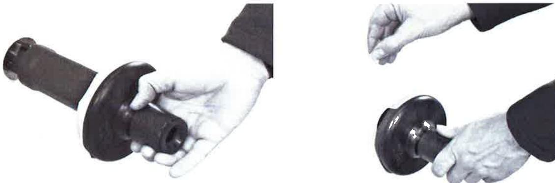
Figure 2. Inserting the universal building entry Hauff MIS60-Dig into the core drill (left) and removing the protective foil of the butyl tape at the rubber flange (right) (pictures of the manufacturer).
